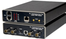
Portable USB based Dual T3 E3 Analyzer Unit (Channelized and Unchannelized T3 E3)
