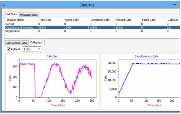
Call Stats provide a running tabular log of system level stats, tracked stats include: Total Calls, Active Calls, Completed Calls, Passed Calls, Failed Call and Instantaneous Calls/Sec.
