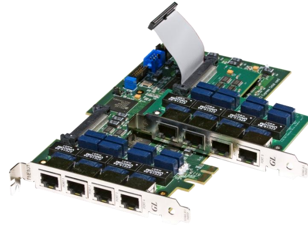
Quad / Octal T1 E1 PCIe Card
