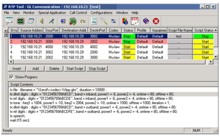
Generation / Detection of in-band and out-of-band digits / tones (DTMF, MF, user-defined, etc.) / events per RFC-2833
