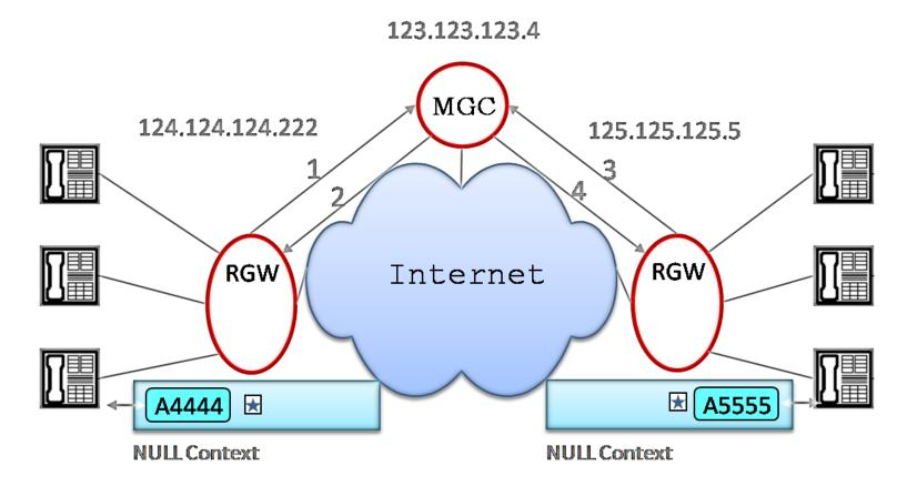
1.(3) ServiceChange(ROOT): MG register with MGC 2.(4) Modify(A4444): MGC set Mode(SendReceive) & Events(al/of)
